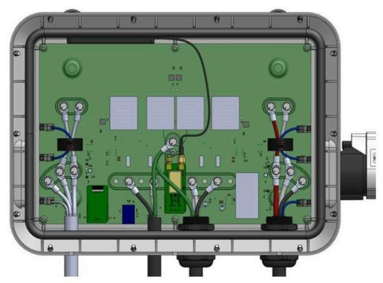
Figure 14: Typical Finished Assembly for 2 Single Phase Feeds
