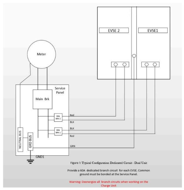
Figure 3:Typical Configuration Dedicated Circuit Dual 50A Unit
