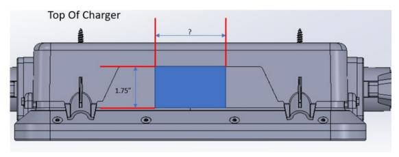
Figure 5: Commercial Charger Label Location
