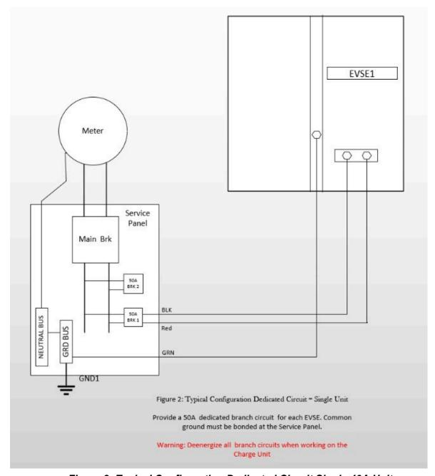
Figure 2: Typical Configuration Dedicated Circuit Single 40A Unit
