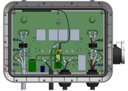
Figure 24: Typical Finished Assembly for 2 Single Phase Feeds
