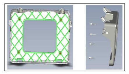
Figure 7: Wall Mounting Bracket Installation
