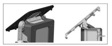
Figure 12: Stowing enclosure cover in cover mounts
