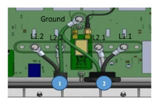
Figure 13: Install Power Leads for Dual Port Configuration
