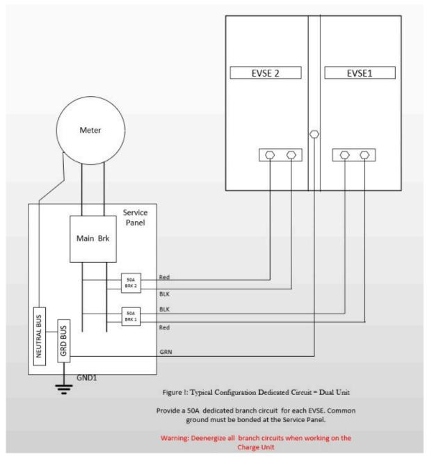
Figure 1: Typical Configuration Dedicated Circuit Dual 40A Unit
