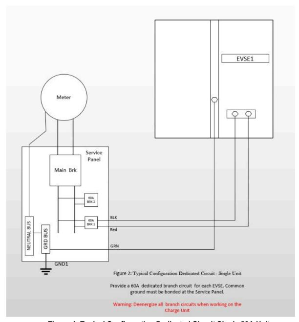
Figure 4: Typical Configuration Dedicated Circuit Single 50A Unit
